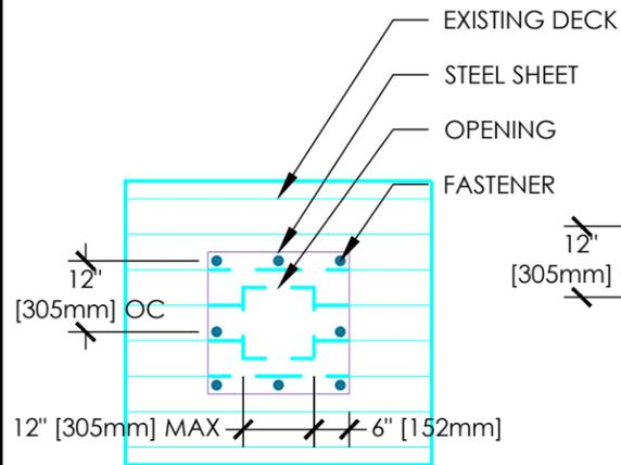
FOR OPENINGS LESS THAN 24" [610mm] BY 24" [610mm]:
